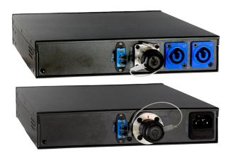
PS-AC100 is a portable power supply unit with compact size and reliable performance. It can provide two 220 VAC outputs totalling 100W over up to 1km of SMPTE cable. With short-circuit protection and load detection and indication, it can meet the requirements of efficient and safe power use in various senarios in live production.
