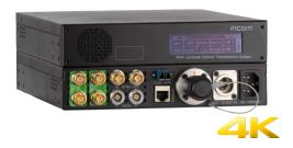
FPT-S2DC is a portable multi-purpose optical transmission device with compact size and reliable performance. With CWDM and TDM techology, it can support two independent 12G-SDI channels, one BB Genlock, two serial communication channels, one gigabit Ethernet and two GPIOs. Equipped OLED screen can display the working status of each channel in real time.
